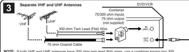
**NOTE:** If both VHF and UHF antennas have 300 ohm twin lead (flat) wires, use a combiner having two 300 ohm inputs and one 75 ohm output.
